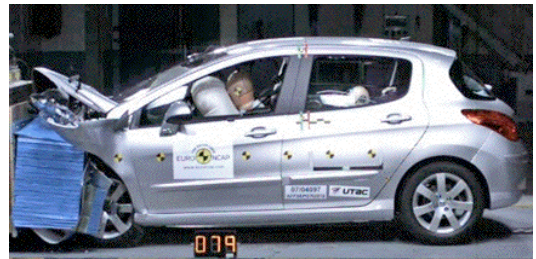
Offset crash test at 64km/h
