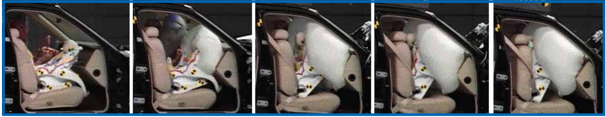
Figure 5 Deployment of a first generation airbag in close proximity to a rearward facing child restraint in the front passenger seating position
